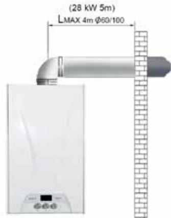
Horizontal Hermetic Flue Application L max. distance with single elbow: 4 m, Ø60/100 L max. distance with single elbow: 6 m, Ø80/125
