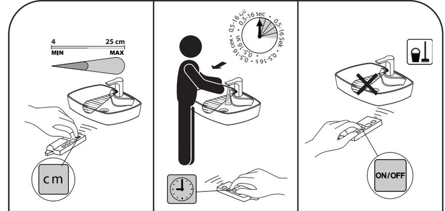
**FR RÉGLAGE DE LA DISTANCE DE DÉTECTION AVEC LA TÉLÉCOMMANDE**
