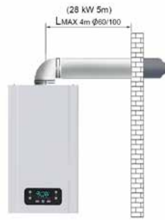
Horizontal Hermetic Flue Application
